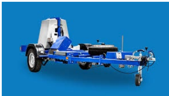
Figure 1 A trailer mounted falling weight deflectometer (left) and a Benkelman Beam and truck set up (right)
